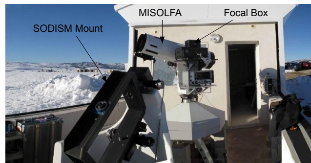
Fig. 1 Picture of MISOLFA monitor and the mount that will receive the qualification model of the PICARD/SODISM telescope at the Calern facility of OCA.
